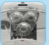
External LED Alley Lights
